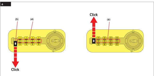
**Opening the combination lock (Figure 5):** Choose the factory-set code 0000 **(4)** or the defined code. Open the lock by turning to the right. The digit wheels are reset to 0000 (to cancel the previous code).
